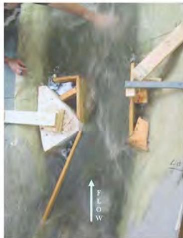
2) Overhead view of the Alternative 4 intake abutments operating at 10,000 cfs. (DMG\_6755)
